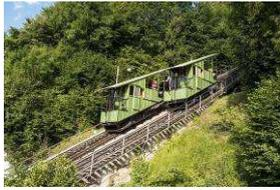
The “Funi” (short for “funicular”) is Switzerland’s last existing water-powered funicular railway and only a few minutes’ walk from the railway station Freiburg. This nostalgic railway has been operating since 1899 – completely without electricity or exhaust fumes. The funicular is not powered by a motor but by residual water from the upper town. It uses filtered waste water from a 3,000-litre tank and thus overcomes 56.4 metres in altitude.
